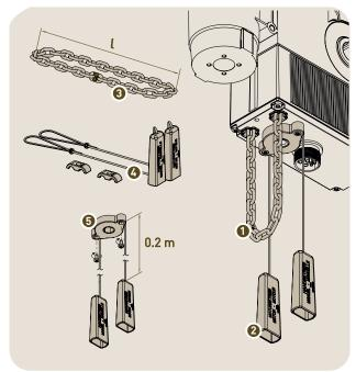
As standard, the drive units have a "rapid hand chain operator SK" with a 4 m long circulating chain (1). Activation takes place using a 0.2 m long shifter cable (2). The following options are possible:
