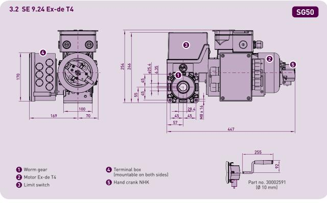
Permitted installation: Horizontal (as shown) or vertical (motor at the bottom or at the top)
