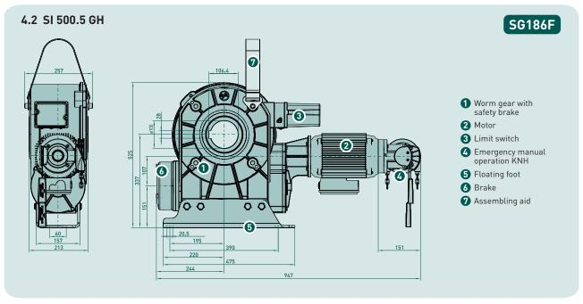
Permitted installation: Horizontal with an additional torque mount system, see 6
